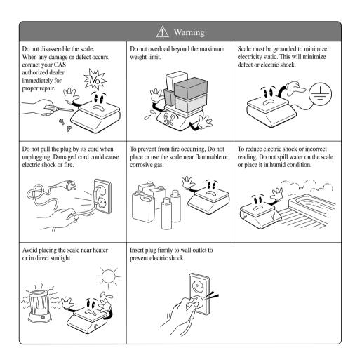
The socket-outlet shall be installed near the equipment and shall be easily accessible. Make sure to plug your scale into the proper power outlet. For maximum performance, plug into a power outlet 30 minutes before the usage for warm up.
