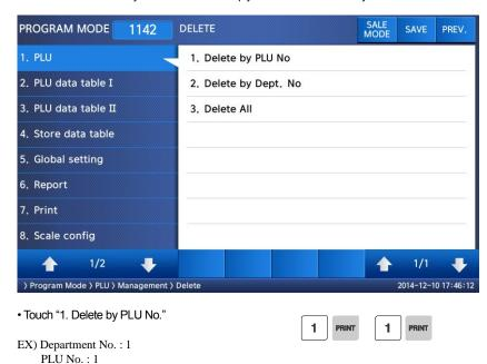
Note: There is no confirmation request for deletion. After entering the PLU number and pressing Print, the PLU will be deleted.
