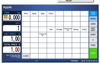
4 Place an item on the platter and press the V1 key.
