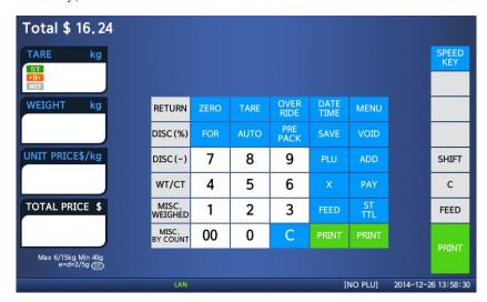
Note: - You can press the VOID key to undo the transaction. (See chapter 3.10).
