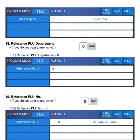
Usage is possible to register the reference key at 1880 in order to use the No. 36~37 reference PLU.
