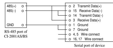
■ Connecting method of RS-485 remote sub display
