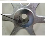
NOTE: TO ENSURE PROPER SAW WHEEL ALIGNMENT, WHEEL MUST BE REINSTALLED ON SAME MACHINE IT WAS REMOVED.
